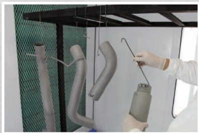
Racking Exhaust Pipes
