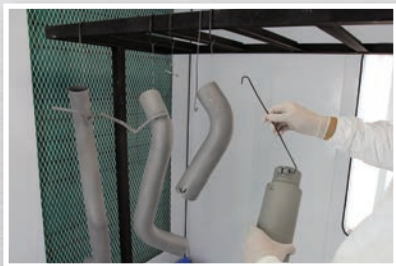
Racking Exhaust Pipes
