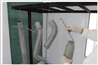
Racking Exhaust Pipes
