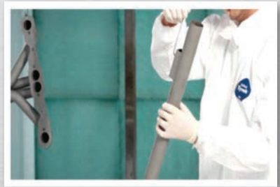
Racking Exhaust Pipes
